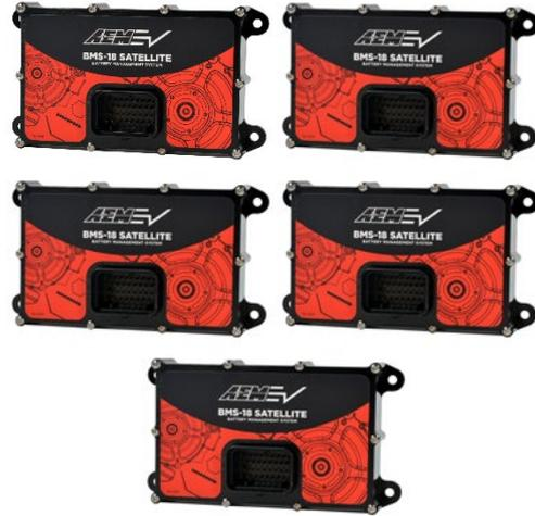
The AEM Battery Management System (BMS-18) hardware expansion for the AEM VCU is a modular BMS add-on designed for multicell lithium battery packs. The BMS allows the VCU to monitor all relevant Battery functions and adds the ability for the VCU to interface directly with a J1772 charging plug and allow the VCU to directly control a supported On-Board Charger (OBC).
